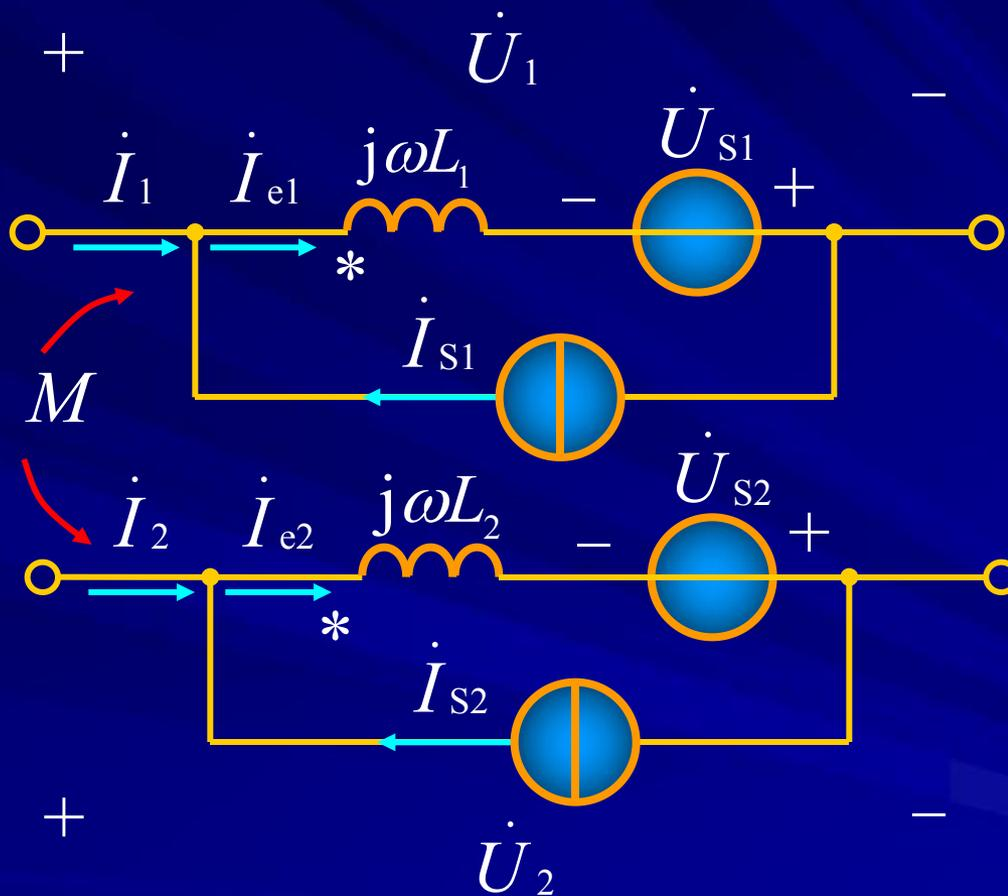
$$[Z_{11}] = \begin{bmatrix} j\omega L_1 & j\omega M \\ j\omega M & j\omega L_2 \end{bmatrix}$$
