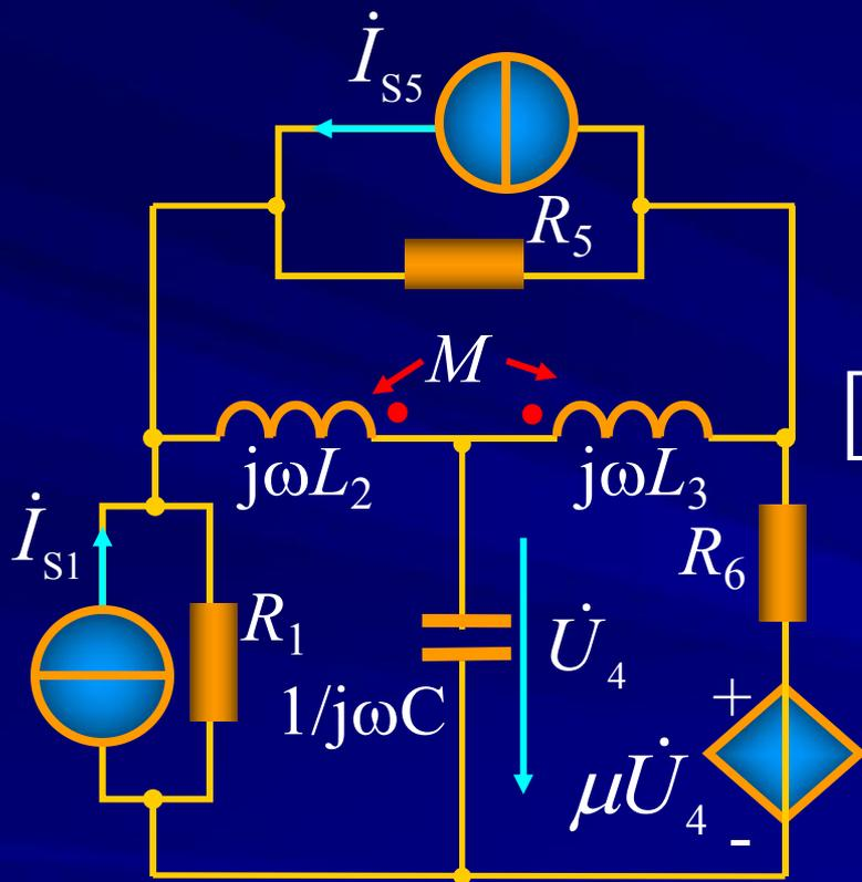
$$[Z] = \begin{bmatrix} R_1 & \dots & & & & 0 \\ 0 & j\omega L_2 \pm j\omega M & & & \dots & 0 \\ 0 & \pm j\omega M & j\omega L_3 & & \dots & 0 \\ 0 & \dots & & 1/j\omega C \dots & & 0 \\ 0 & \dots & & \mu/j\omega C & R_5 & 0 \\ 0 & \dots & & & & R_6 \end{bmatrix}$$
