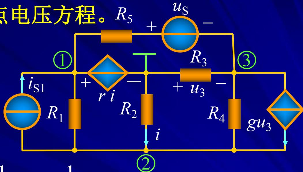
$$\begin{cases} u_{n1} = ri \\ \left(\frac{1}{R_1} + \frac{1}{R_2} + \frac{1}{R_4}\right)u_{n2} - \frac{1}{R_1}u_{n1} - \frac{1}{R_4}u_{n3} = -i_{S1} + gu_3 \\ -\frac{1}{R_5}u_{n1} - \frac{1}{R_4}u_{n2} + \left(\frac{1}{R_4} + \frac{1}{R_3} + \frac{1}{R_5}\right)u_{n3} = -gu_3 - \frac{u_S}{R_5} \end{cases}$$
