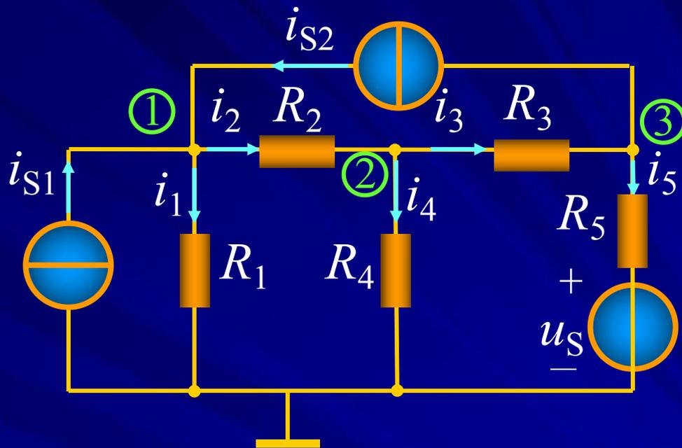
$$\begin{cases} \frac{u_{n1}}{R_1} + \frac{u_{n1} - u_{n2}}{R_2} = i_{S1} + i_{S2} \\ -\frac{u_{n1} - u_{n2}}{R_2} + \frac{u_{n2} - u_{n3}}{R_3} + \frac{u_{n2}}{R_4} = 0 \\ -\frac{u_{n2} - u_{n3}}{R_3} + \frac{u_{n3} - u_S}{R_5} = -i_{S2} \end{cases}$$
