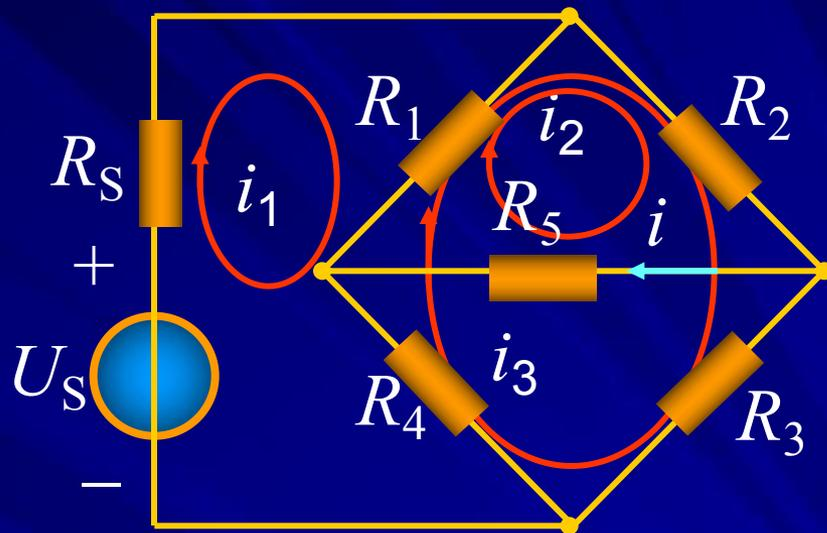
$$(R_S + R_1 + R_4)i_1 - R_1i_2 - (R_1 + R_4)i_3 = U_S$$
