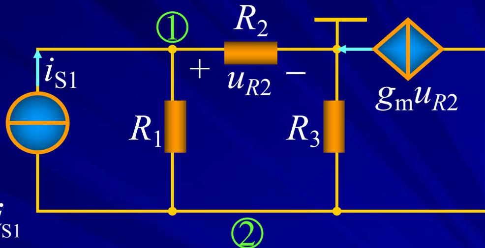
$$\begin{cases} \left(\frac{1}{R_1} + \frac{1}{R_2}\right)u_{n1} - \frac{1}{R_1}u_{n2} = i_{S1} \\ -\frac{1}{R_1}u_{n1} + \left(\frac{1}{R_1} + \frac{1}{R_3}\right)u_{n2} = -g_m u_{R2} - i_{S1} \\ u_{R2} = u_{n1} \end{cases}$$
